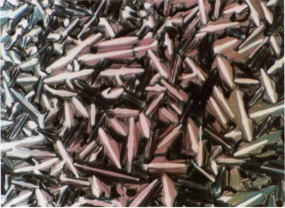
Figure 3. A8: Optical texture of the liquid crystal phase at 430 K on cooling. Crossed polarizers.
